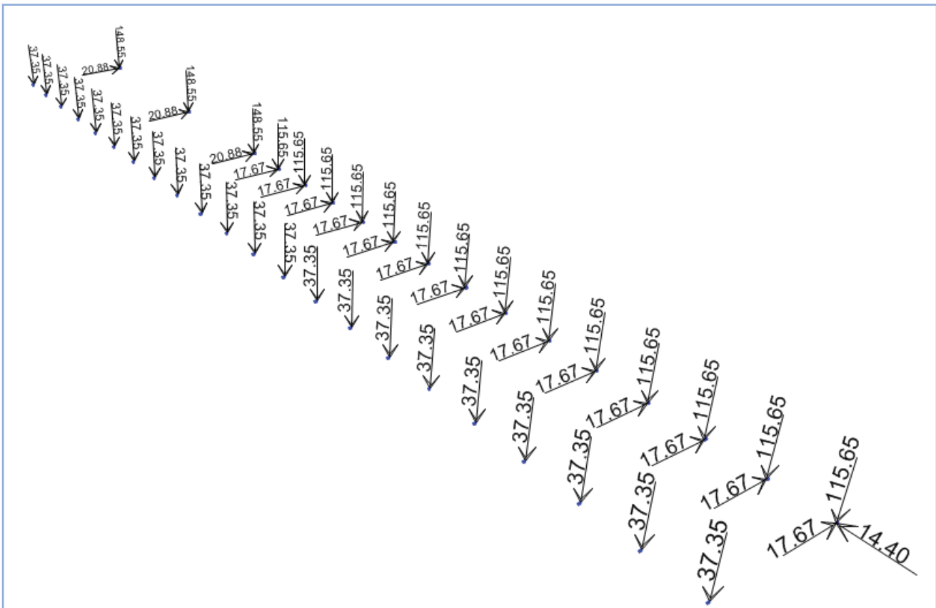
Figure 4 95 Crane load 2 (CR2)
