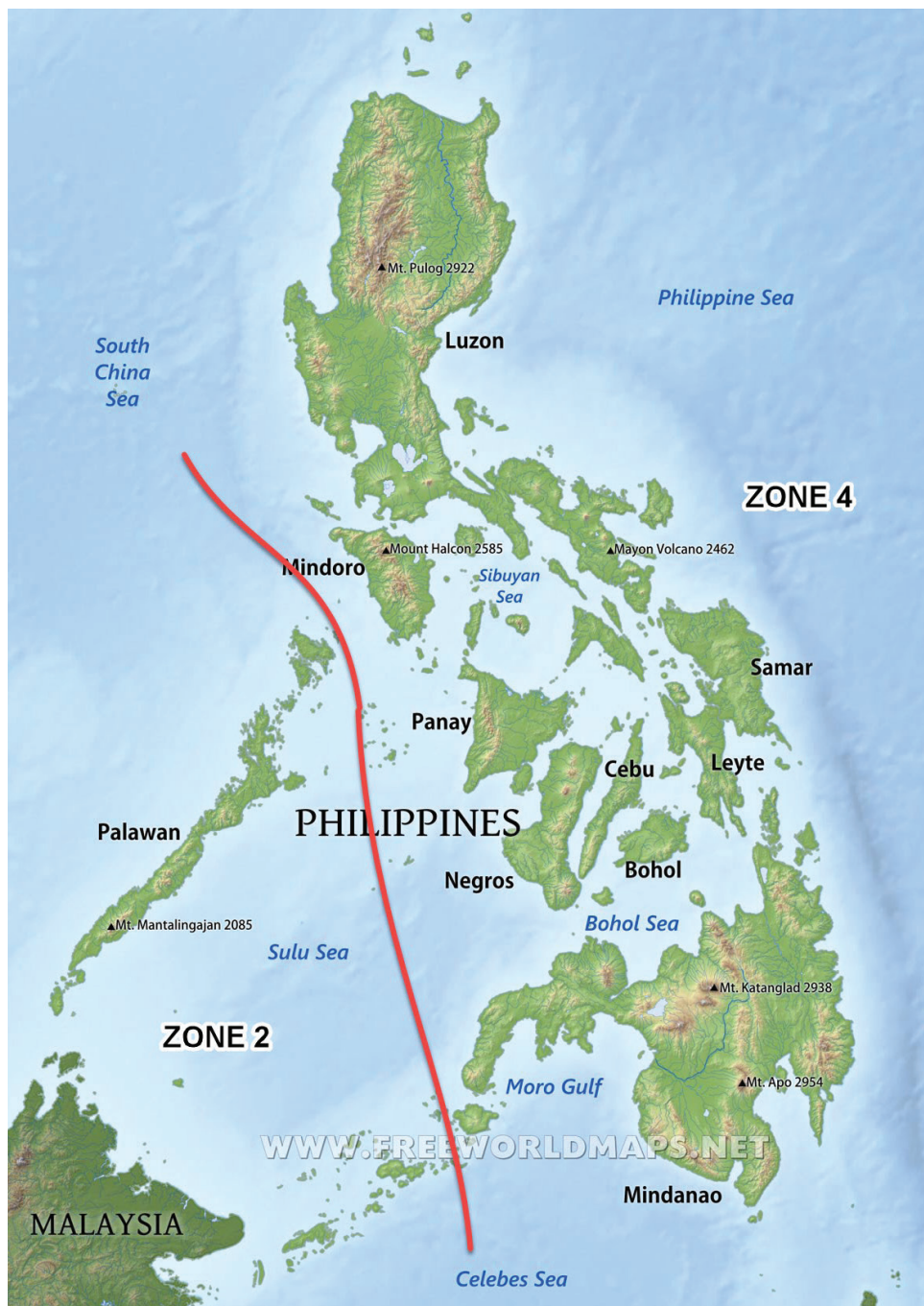
Figure 2.9 Philippines Seismic zones map with 500-year return period (Figure 208-1 NSCP 2015)
